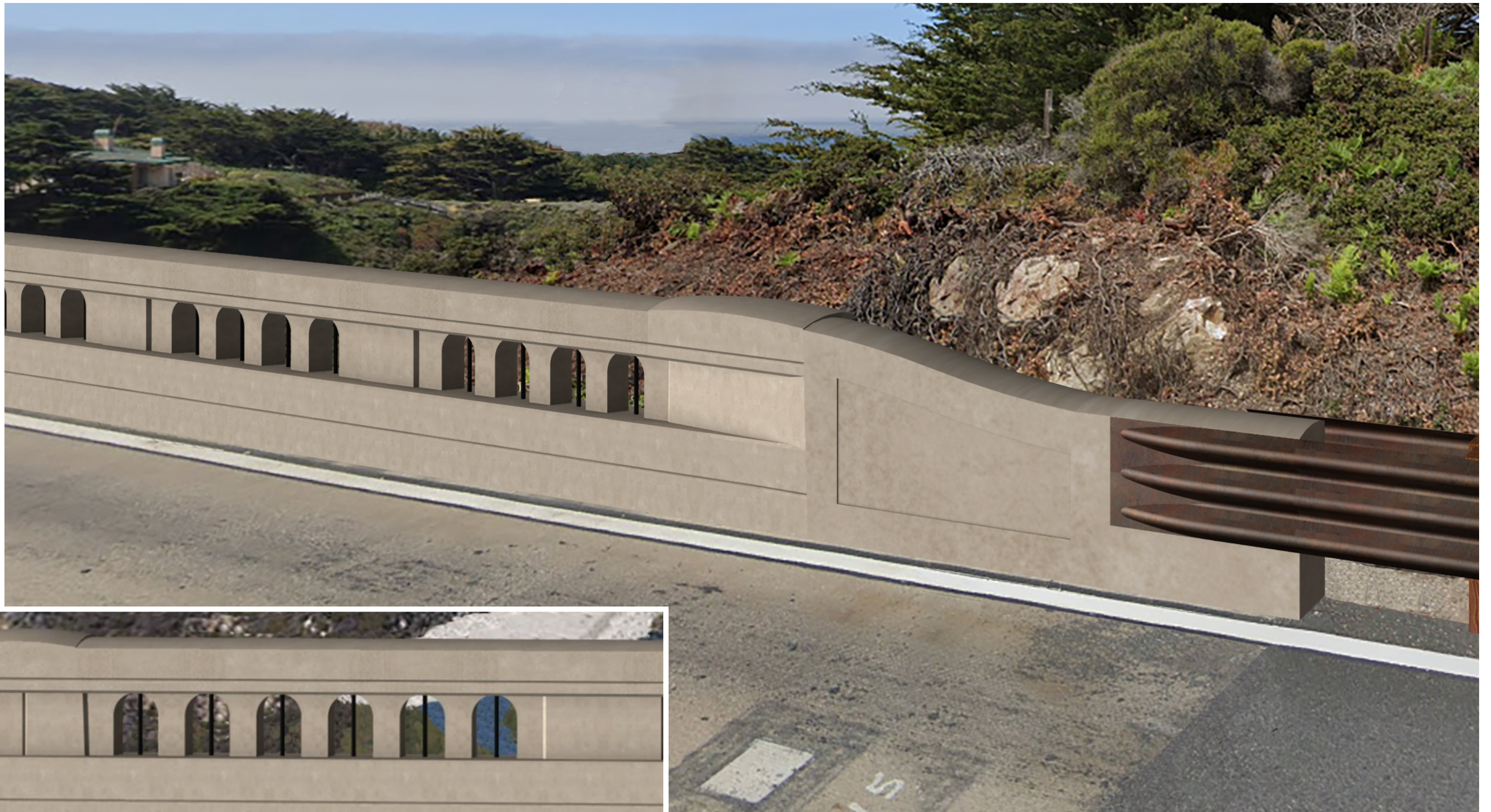
Barrier Alternative - 4A 10" Clear Opening with Dark Single Bar
