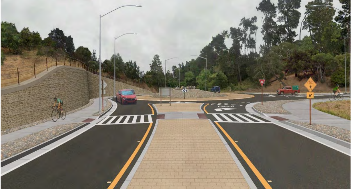
Figure 2.1.10.8 Alternative 1 Hardscaped Roundabout
