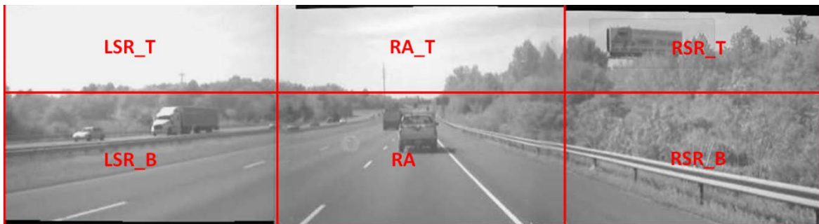
Figure 9. Screen capture showing static ROIs on a scene video output.
