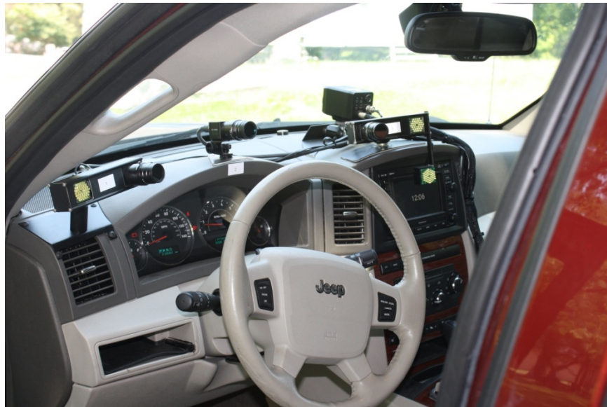
Figure 1. Eye tracking system camera placement.
