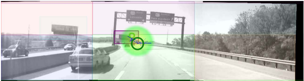
Figure 21. Heat map near the middle of a DCZ for a standard billboard in the daytime on a freeway.
