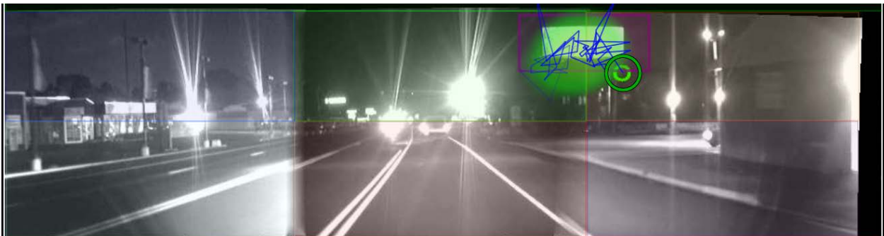
Figure 16. Heat map near the end of a DCZ for a standard billboard at night on an arterial.
