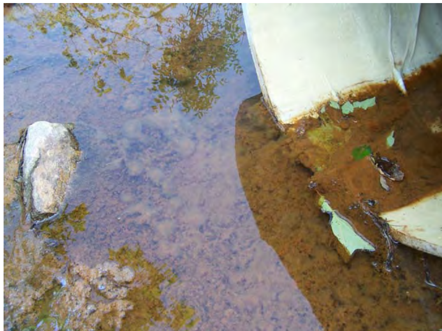
Figure 3. Algal blooms at Site 3, photographed 24 days after installation. Algal blooms appeared within 6 to 8 days after installation at Sites 1, 2, and 3 and were present up to 8 in below water surface near pipe outlet and up to 50 m downstream.
