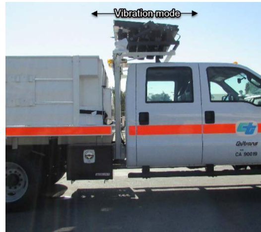
Figure 1: Apparent direction of forces causing potential failure of cantilevered structure attached behind cab.
