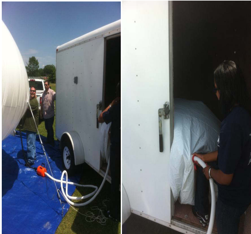
Figure 11. Transferring Helium from Balloon to Bladder
