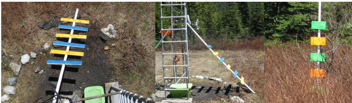
Figure 7. Aerial snow markers deployed at Snoqualmie Pass tower.
