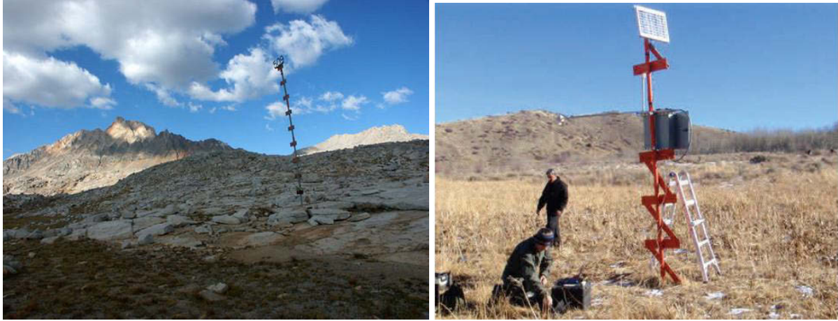
Figure 2. (left) Aerial snow depth marker in Humphreys Basin (near Cony Lakes and Mt. Humphreys) (from http://www.summitpost.org/aerial-snow-depth-marker-in/28710 ) (right) Aerial marker in Utah with iridium technology (Julander 2012).
