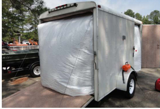
Figure 12. Helium stored in bladder
