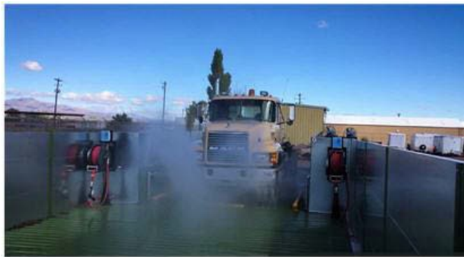
Pre-Wash Spray Bars on Pre-Wash Section
