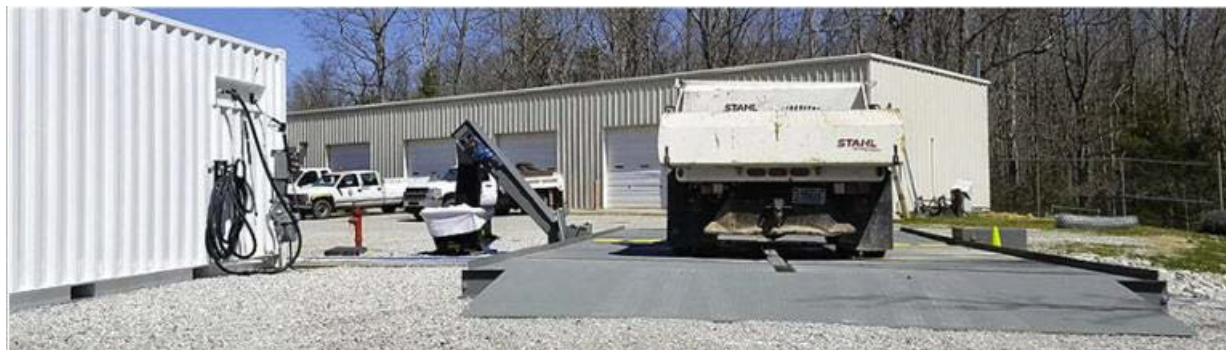
Figure 8. EST Co. Wash Rack System Shown with Mud Conveyor, Pressure Washer Wands, and Filter System HE Hydro Engineering, Inc.
