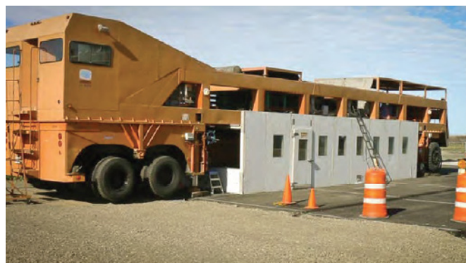
Figure 1: Heavy Vehicle Simulator used for testing
