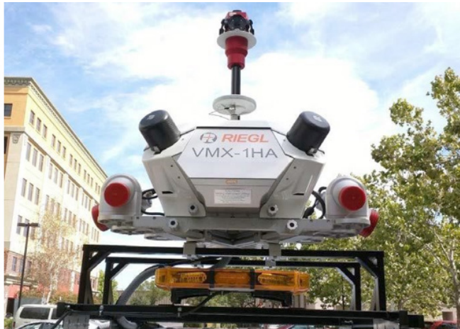
Image 2: Riegl VMX-1HA sensor pod mounted on a Caltrans vehicle
