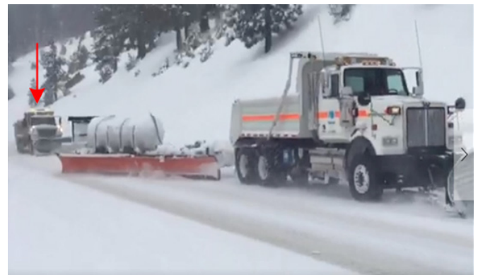
Figure 1: Additional Sander Truck Trailing TowPlow on I-80
