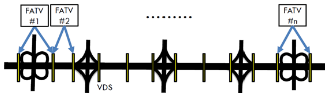
Image 5: Point Detector Placement Strategy. Select point detectors representing a single Fully Accounted Traffic Volume (FATV) group. Study impacts on performance measures of each detector group by removing the group
