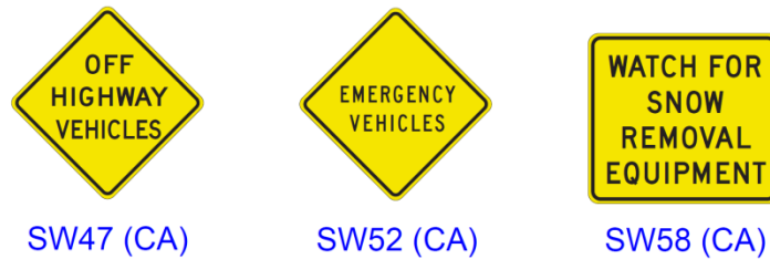
Figure 2C-10 (CA). Vehicular Traffic Warning Signs and Plaques
