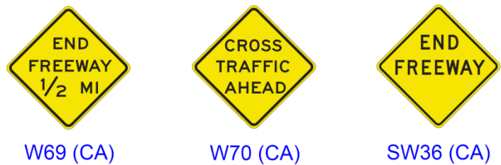
Figure 2C-9 (CA). Intersection Warning Signs and Plaques
